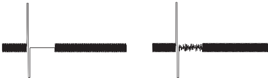
Fig. 3. (Left) Artificial data created to simulate a typical CSP. (Right) The same artificial data with white noise added to the CSP interval.
